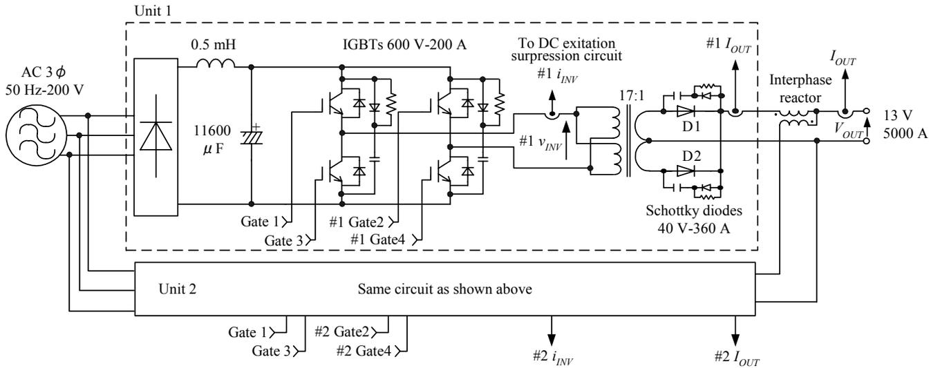
Fig. 2. Schematic diagram of 13-V, 5000-A DC power supply.
