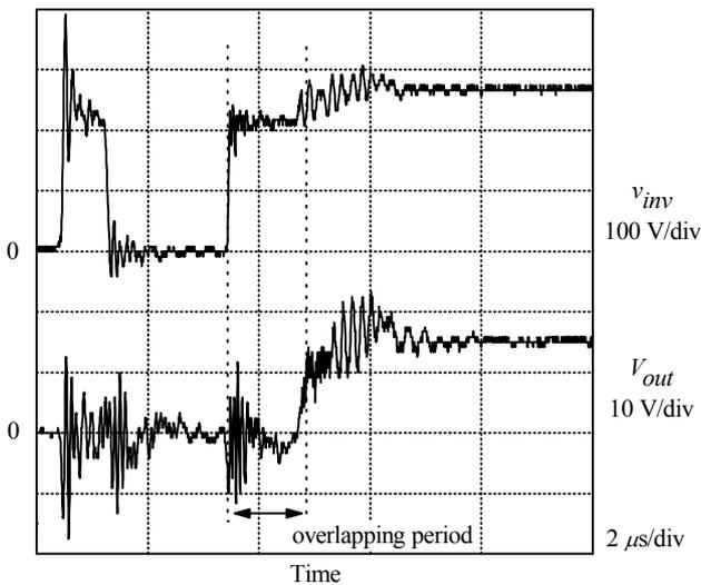
Fig. 12. Waveforms of overlapping period in commutation.
