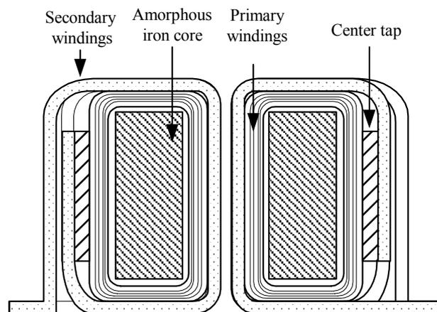
Fig. 5. Cross section diagram of high-frequency step down transformer.
