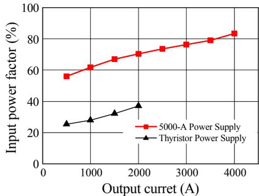
Fig. 10. Total input power factor on utility power source side.
