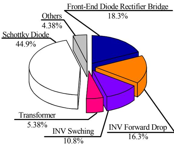
Fig. 11. Loss analysis result at 80% (4000-A) load.
