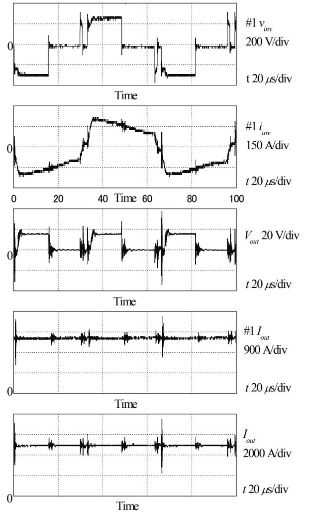
Fig. 8. Waveforms of 15-kHz inverter and output DC bus.
