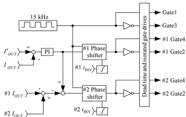
Fig. 4. Block diagram of 13V-5000A DC power supply controller.
