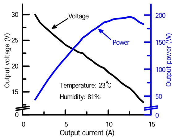
Fig. 4. Characteristics of the PEM fuel cell.
