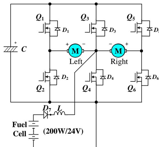
Fig. 6. Improved three-leg full-bridge DC chopper with boost function.
