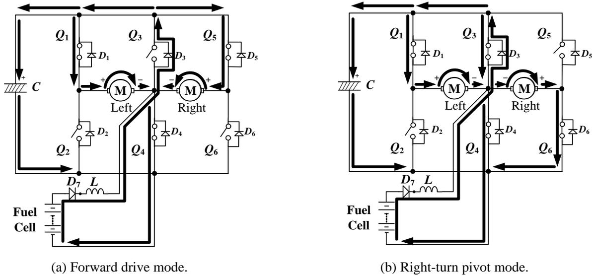
Fig. 7. Basic operations of the improved three-leg full-bridge DC chopper.
