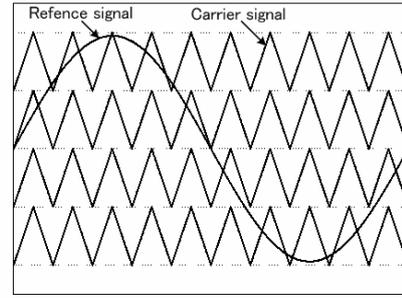
Fig. 13. Multi-carrier based sinusoidal PWM
