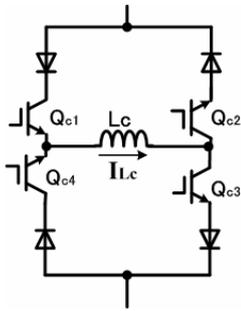
Fig. 3. Proposed inductor-cell circuits
