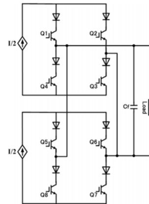
Fig. 1. Five-level paralleled H-Bridge CSI
