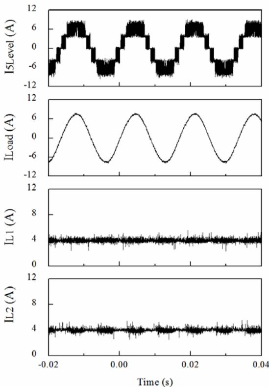
Fig. 16. Experimental waveforms of five-level DC-current module type CSI
