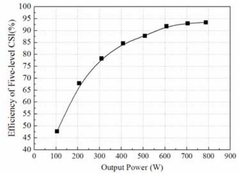
Fig. 18. Efficiency characteristics of five-level DC-current module type CSI
