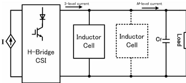
Fig. 4. Proposed  $M$ -level inductor-cell type CSI
