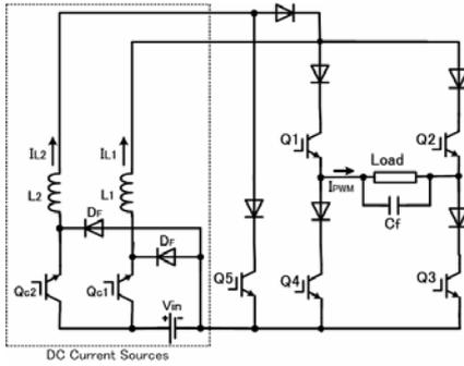
Fig. 11. Five-level DC-current module type CSI with chopper based DC current-sources
