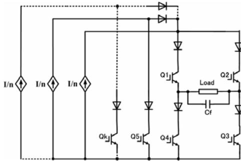
Fig. 8. Proposed  $M$ -level DC-current module type CSI
