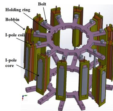
Fig. 12. Mechanical configuration of I-pole unit.
