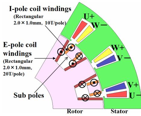
Fig. 1. Cross section diagram of proposed motor.
