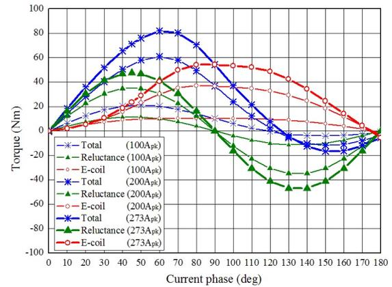
Fig. 6. Current phase-torque characteristics at 1000 r/min.
