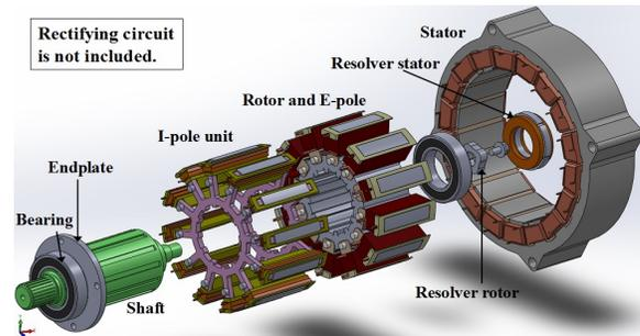
Fig. 14. Mechanical configuration of proposed motor.
