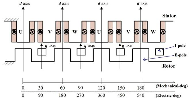
Fig. 3. Developed salient pole model of proposed motor.
