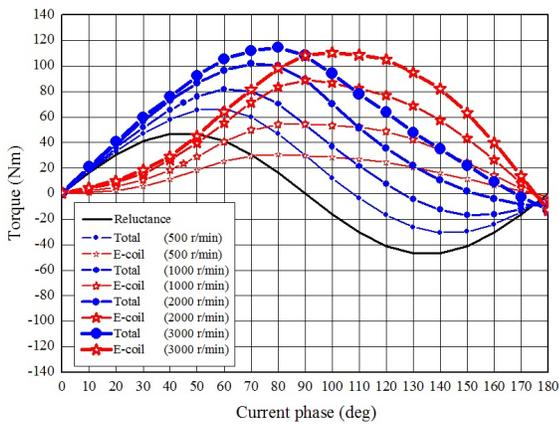
Fig. 9. Current phase-torque characteristics at 273 A<sub>pk</sub>.
