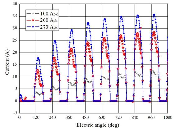
Fig. 7. Induced current characteristics at 1000 r/min.
