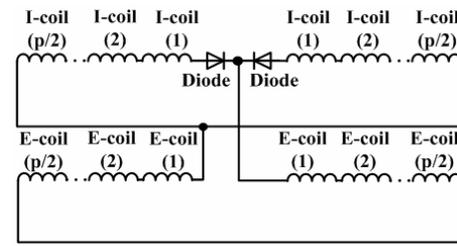
Fig. 2. Rotor winding connection diagram using full-bridge rectifier.
