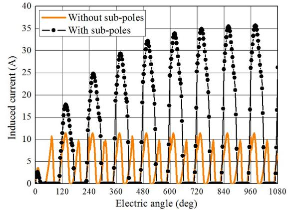
Fig. 5. Induced current waveforms in forward direction.
