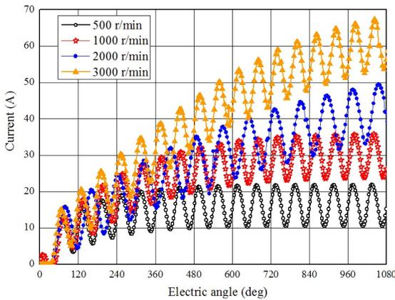
Fig. 11. Field current characteristics at 273 A<sub>pk</sub>.
