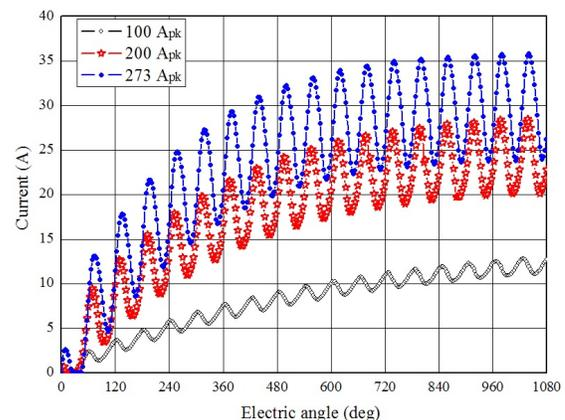
Fig. 8. Field current characteristics at 1000 r/min.
