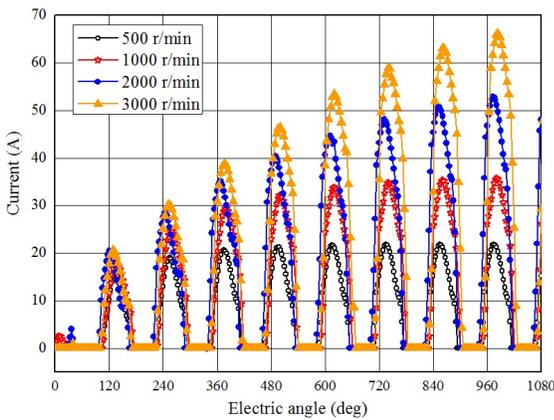
Fig. 10. Induced current characteristics at 273 A<sub>pk</sub>.
