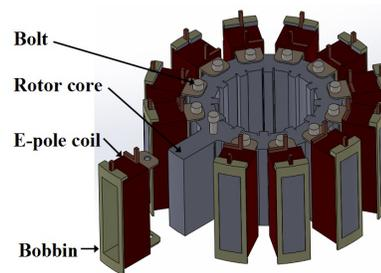
Fig. 13. Mechanical configuration of rotor and E-pole.
