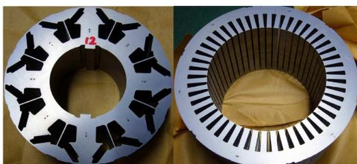
(c) Motor cores of benchmark IPMSM.
