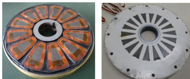
(a) Wound-field rotor with resin mold.
