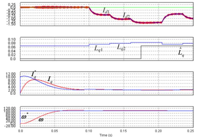
Fig. 5. Simulation result of  $L_q$  identification.
