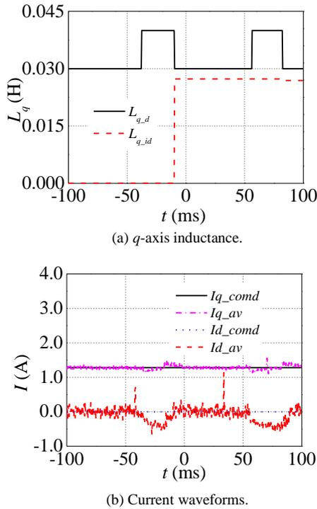
Fig. 8. Experimental result of  $L_q$  identification with extra  $R$ .
