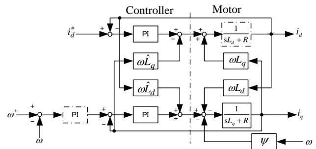
Fig. 1. Field-oriented control system of IPM motor.
