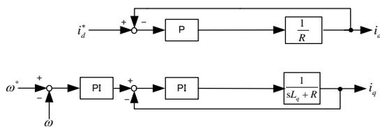
Fig. 9. Simplified  $R$  identification system.
