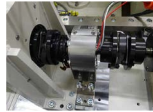
Fig. 8. Slip-ring for rotor current measurement.
