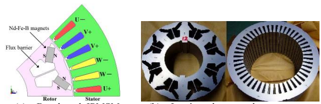
(a) Benchmark IPMSM. (b) Laminated rotor and stator core. Fig. 20. Benchmark IPMSM with Nd-Fe-B magnets.
