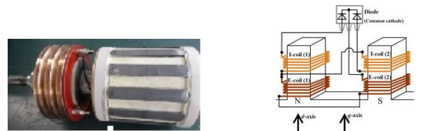
(b) Benchmark model with slip-ring. (c) Rotor winding connection diagram of benchmark.
