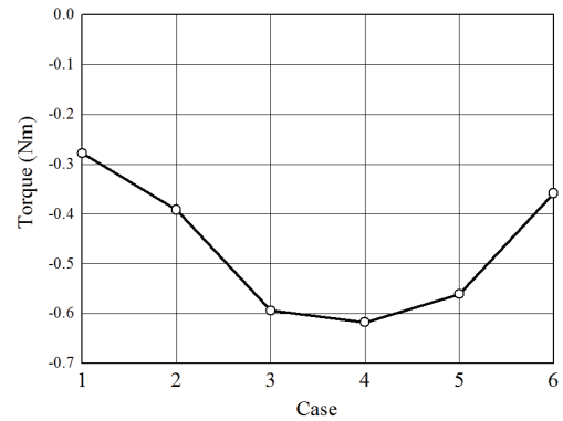
Fig. 10. Regenerating torque characteristics with respect to induction rotor winding configuration under 389 A rms T and s_1 = 0.3 in case of 24-rotor slots.
