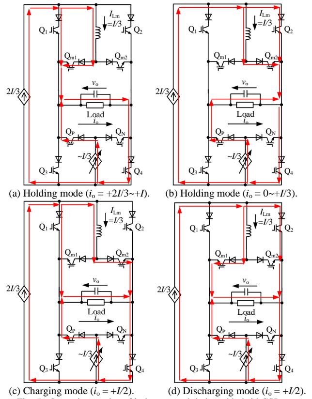
Fig. 5. Operation modes of inductor module based hybrid CSI.
