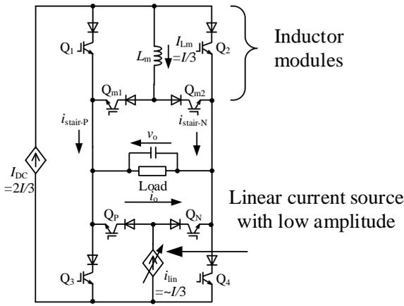
Fig. 3. Proposed hybrid CSI with inductor module.
