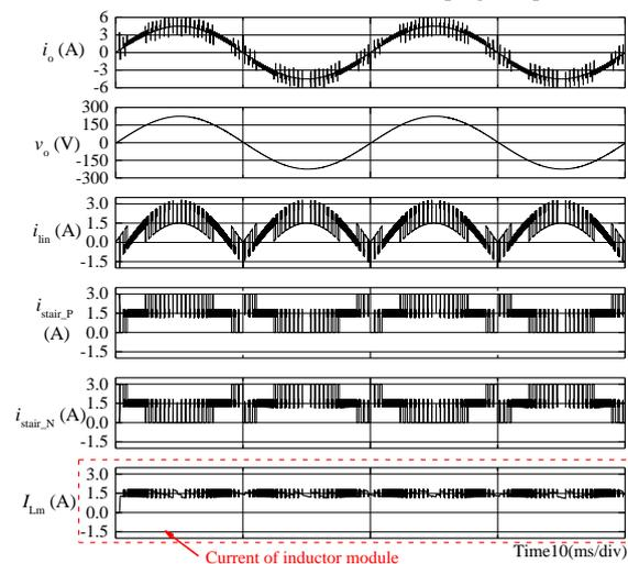
(b) Waveforms with inductor current drooping compensation.
