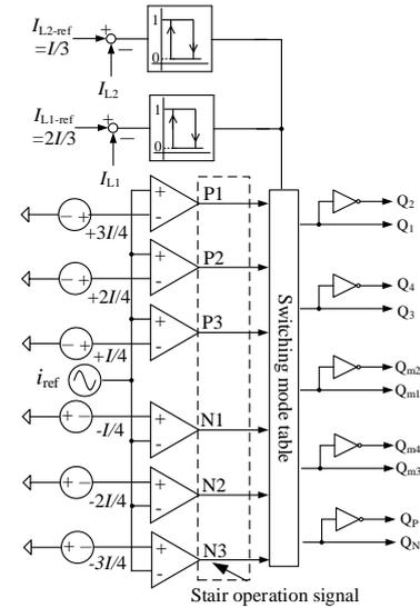
Fig. 13. Control block diagram of 7-level main CSI.
