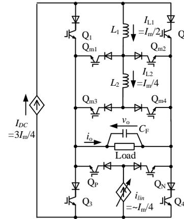
Fig. 12. Inductor module based 7-level hybrid CSI.
