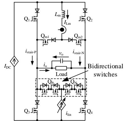
Fig. 15. Inductor module based hybrid CSI with bidirectional switches
