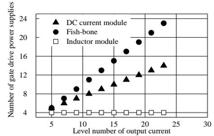
(c) Output levels and gate drive power supply counts.
