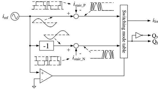
Fig. 10. Control block diagram of variable current source.
