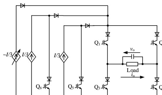
Fig. 1. Hybrid CSI with DC current source modules.
