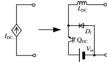
Fig. 6. Chopper based DC current source.
