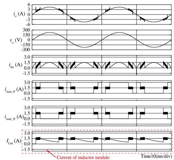
(a) Waveforms without inductor current drooping compensation.
