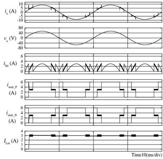
Fig. 11. Simulation waveforms of proposed 5-level hybrid CSI.
