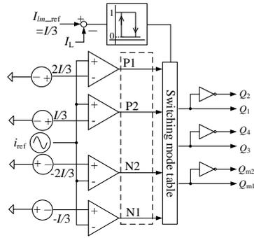
Fig. 9. Control block diagram of 5-level main CSI.
