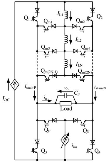
Fig. 7. Generalized multilevel inductor module based hybrid CSI.
