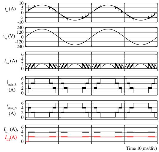
Fig. 14. Simulation waveforms of proposed 7-level hybrid CSI.
