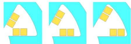
Fig. 2. Analysis model with slot depth modification.
